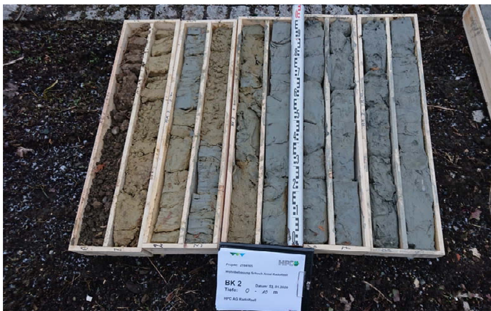
Foto 7: Bohrkern BK 2, 0 – 10 m
