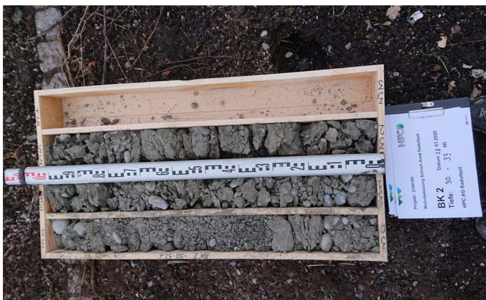
Foto 10: Bohrkern BK 2, 30 – 33 m
